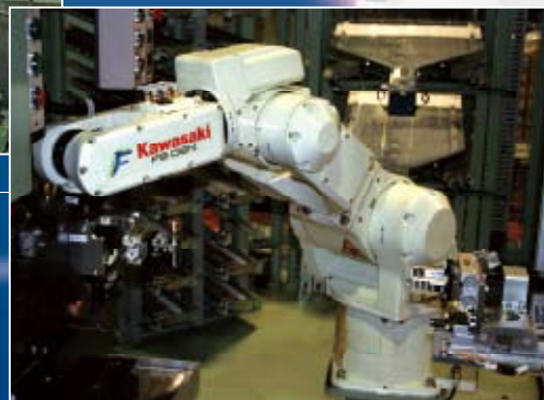
Caulking work of oil hydraulic pump
