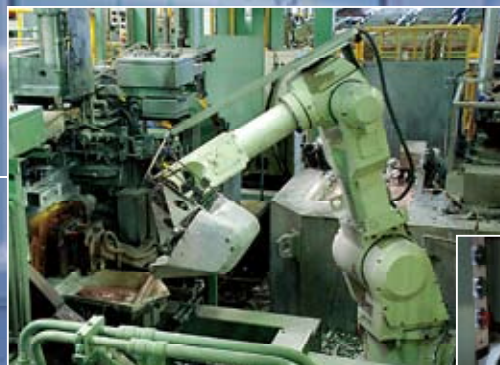
Molten aluminum ladling process work for aluminum casting parts
