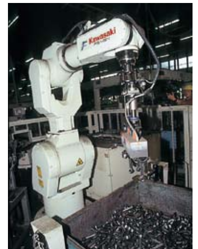
Depalletizing system of connecting rod
