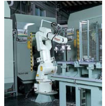
Handling of small-size engine case
