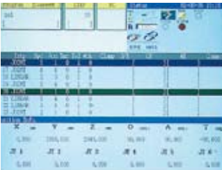
Teaching Screen Simplified Operation (Block) teaching system by block selection
