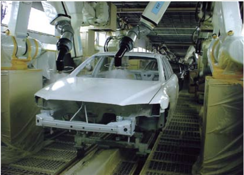
Automobile body coating line Photo : Mazda's 3 wet-on coating system clear coating process
